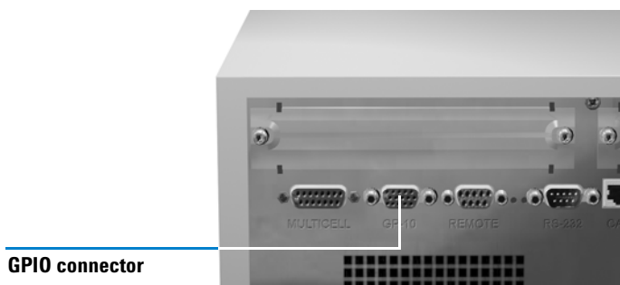
Figure 18 GPIO Connector at Rear of the Spectrophotometer
